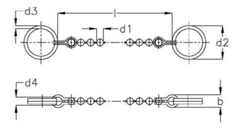
$\begin{array}{lll} b & = 6 \\ d1 & = 3.5 \\ d2 & = 14 \\ d3 & = 1.0 \\ d4 & = 4 \\ I & = 1000 \\ Static load (N) = 50 \end{array}$
